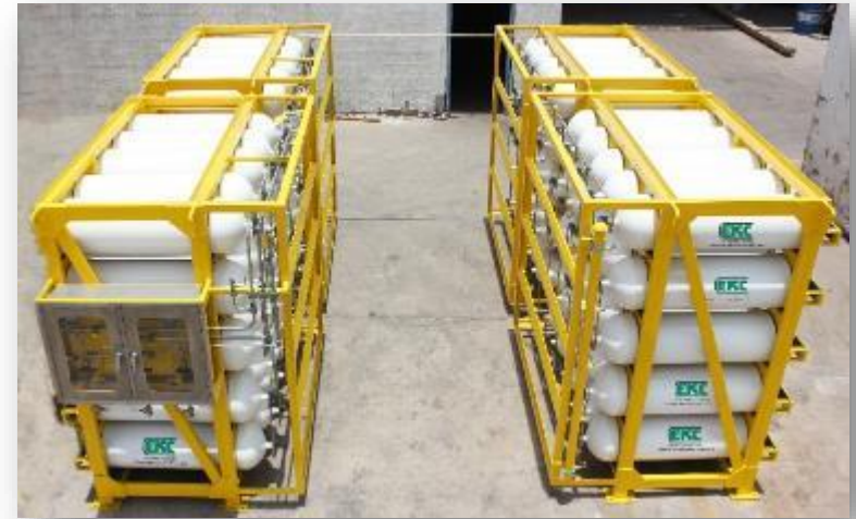
STORAGE CASCADE FOR CNG STATIONS
